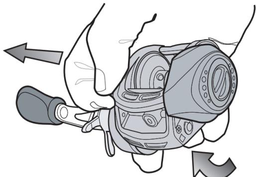
2. TO OPEN, rotate palming sideplate up.
